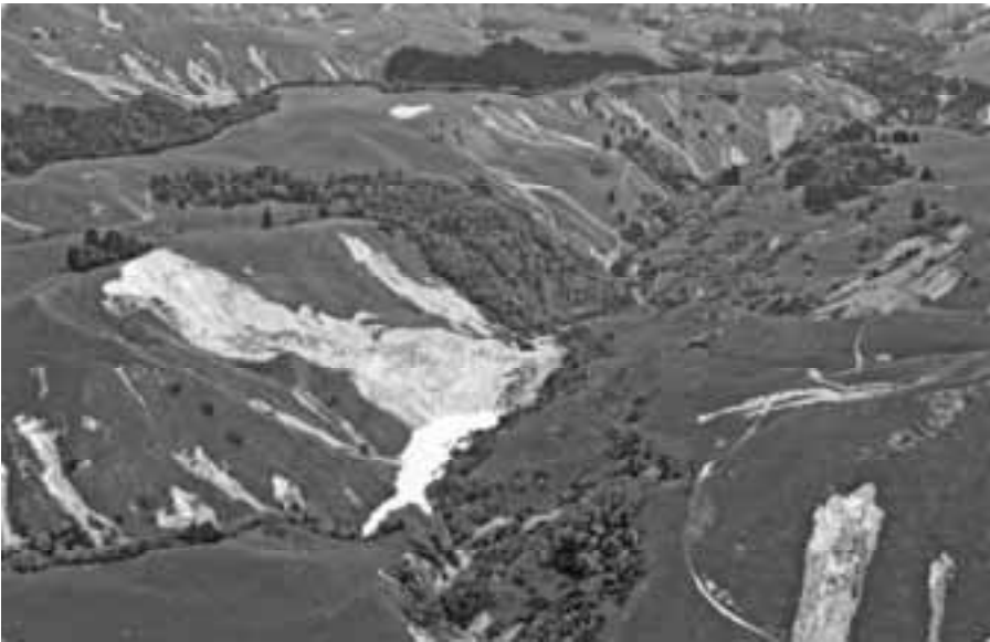
Plate 19: Large slump in the Whangaehu catchment. Also note the surrounding soil slip erosion (IGNS).
