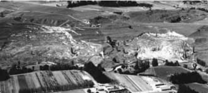
Plate 16: Slump erosion, Dannevirke (NT). Note the rotation across the back-wall. Some flow characteristics have developed after the initial slump failure.
